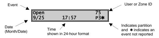
This screen shows an opening of Partition 3 on September 25<sup>th</sup> at 5:27 p.m. by user 75. The [\*] shows that this event is not programmed to be reported to the central monitoring station.
